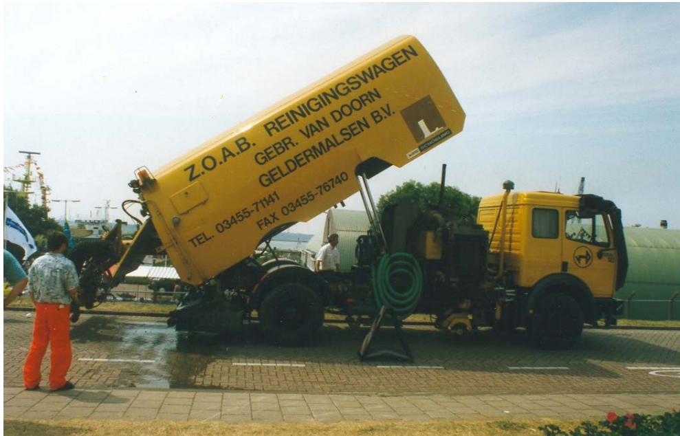
FIGURE 6 PFC (ZOAB in Dutch) cleaning machine.
