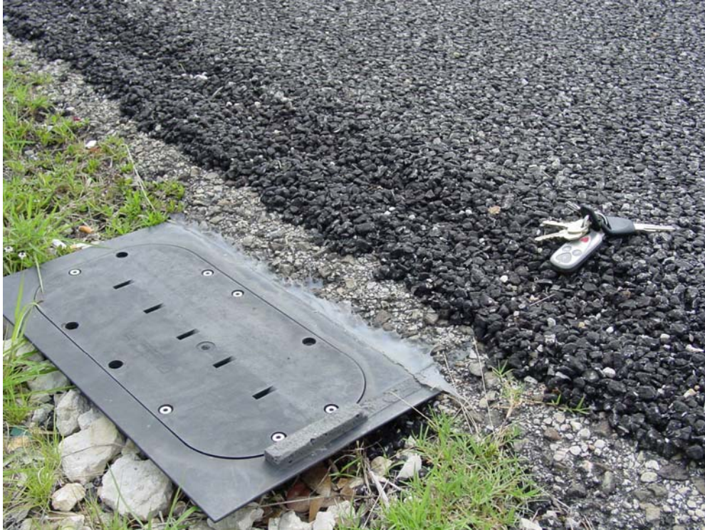
FIGURE 2 Photograph of installed sampler at edge of pavement.
