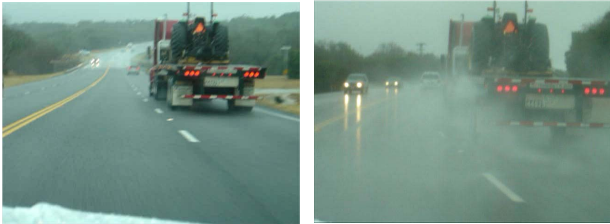
FIGURE 1. Difference in Spray from Conventional and PFC Pavements
